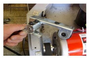
5. Remove the 2 screws holding the front roller in place.
