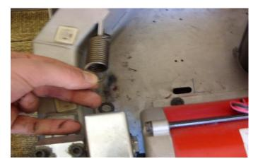
3. Remove the top plate of the tension wheel set. The top plate can be discarded, it will not be re-used.
