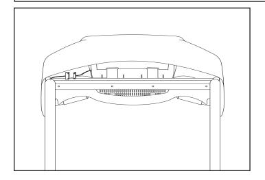
1. Connect the console cable. Carefully tuck wires in mast to avoid damage.
