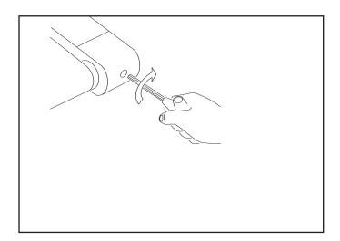
**CENTERING THE RUNNING BELT** (NOTE: Running belt should NOT be moving during adjustments) **If the running belt is too far to the right side:** turn the right adjustment bolt clockwise 1/4 turn at a time. Turn the treadmill on and check the belt alignment. Repeat if necessary, until the belt remains centered during use (using the supplied Allen wrench).
