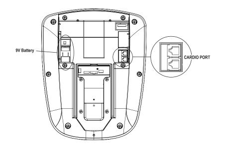
**BATTERY**: Your console is equipped with a 9V battery to maintain workout information.
