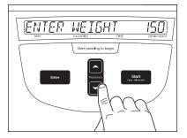
The WATTS programs will ask you to set the desired WATT level instead of resistance levels. The WATT level will range from 40 to 250 in increments of five.
