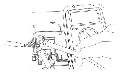
To check the voltage of a specific function (i.e. elevation, motor control, etc), place the negative lead of your multi-meter on pin B3, B4 or B5, and place the positive lead on the desired pin. Follow the voltage charts on p23 (9wire) and p24 (12wire).
