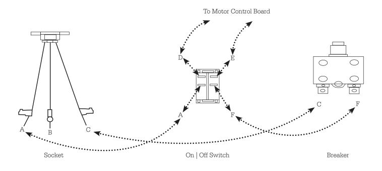
A – Socket wire to breaker or on/off switch.
