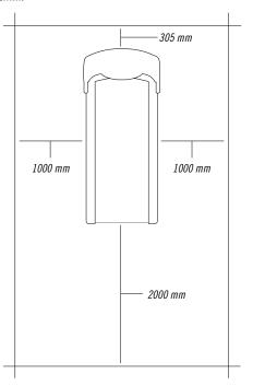
Please leave a 78.75" (2000 mm) x 39.50" (1000 mm) landing zone behind the treadmill. This zone is to allow easy access to the treadmill and gives the user an easy exit path from the machine. In case of an emergency, place both hands on the side arm rests to hold yourself up and place your feet onto the side rails.
