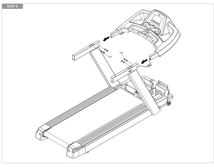
Connect the console cables from the console set to the motor control board cables. Secure the console set with 2 screws (Z52) on each side.
