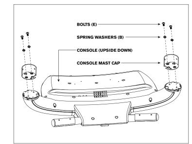
NOTE: The console mast caps are marked with an L if they are to be used on the left-hand side of the treadmill or an R if they are to be used on the righthand side of the treadmill. If the console mast caps are assembled on the incorrect side of the treadmill,
