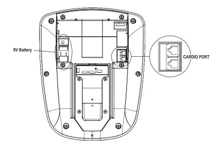
**BATTERY**: Your console is equipped with a 9V battery to maintain workout information.
